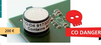
This sensor is optionally built into Nesis and it is able to give you an early warning of this lethal gas.
